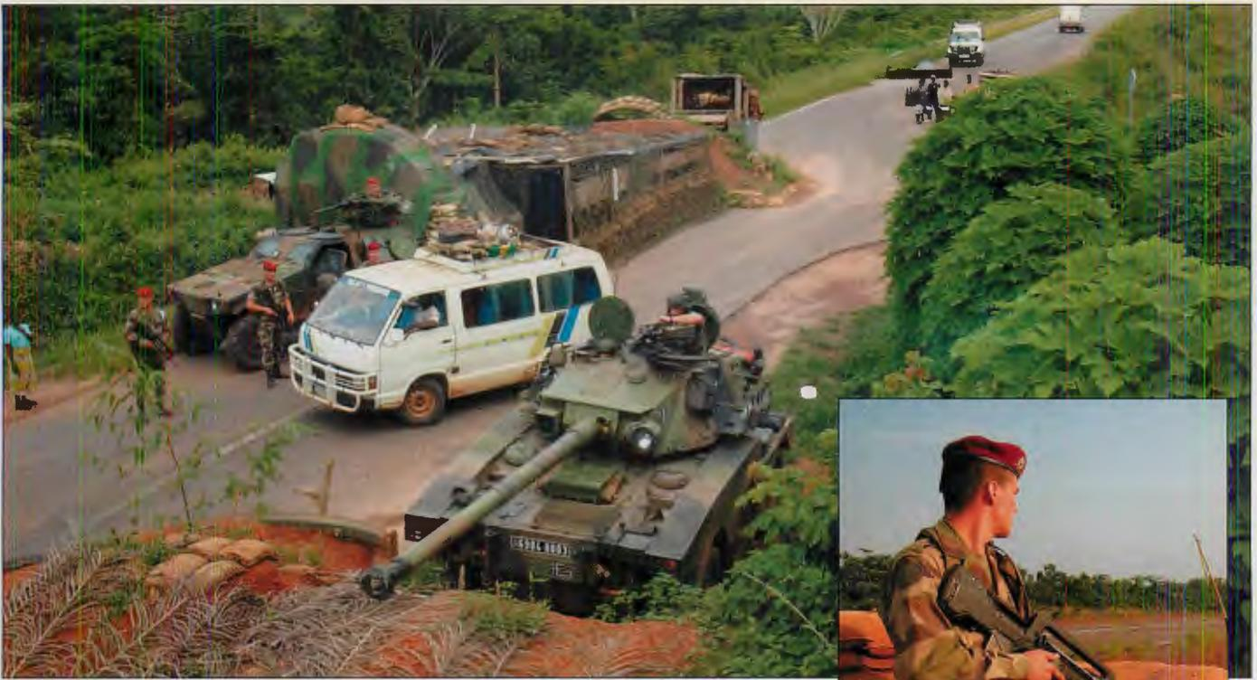
*Roadblocks established on each side of the "zone of confidence" help keep warring factions apart, and stem the infiltration of hostile men and materiel. The Sagai RC-90 light tank, which mounts a 90mm gun, has proved heavy enough to get the job done on such peace-keeping missions, yet light enough to get to where the job is. (inset) French trooper with FAS rifle stands watch on the small air strip near the city of Man.*
